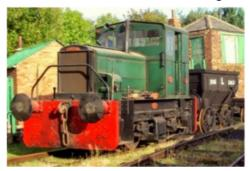
The Bowes loco, photo above right, is works number 3922 built in 1959 and spent its working life with the NCB Durham collieries in the local area. With the decline of coal mining in the 1970's she was surplus to requirements and was acquired by the Bowes Railway in 1979. The loco was built with a Dorman 6KD engine, a 6 cylinder diesel developing 168hp.
