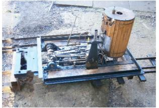
With the body panels removed we can see the Chaloner boiler (coal fired, of course) mounted in front of the twin cylinder power unit. These are standard Chaloner cylinders with the piston valve chests in between. They are mounted horizontally with the crankshaft further back on the chassis.
