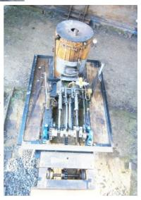
Steam is taken from the top of the boiler and fed to the cylinders via a simple ball valve regulator. The exhaust steam is piped from the bottom of the valve chest, up the outside of the boiler before entering the smokebox area with a blast nozzle directing the exhaust up the centre chimney. Extension tubes are fitted to the exhaust and safety valve vent terminating just above the cab roof.
