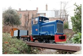
Talking of Planets, we have had a bit of a revamp on the 7½" gauge Planet 2 design. A new chassis with outside frames means we can now offer this loco in 5" gauge and as a petrol hydraulic, like the old Simplicity 2. The electric version has a new geared motor, one to each axle giving over 600 watts of power. The body and detailing are the same as the earlier version of this popular loco.
