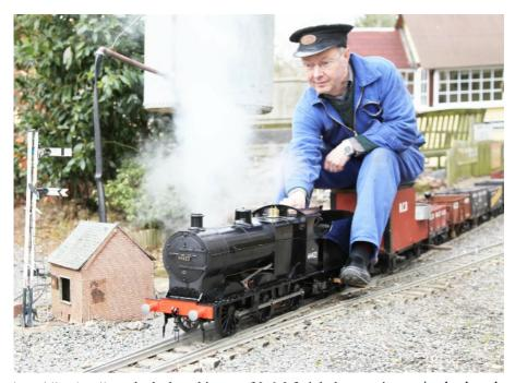
The Midland Railway had a long history of 0-6-0 freight locomotives going back to the Victorian period, the final version of the locomotive type was the Fowler designs 4F. The first example was built in 1911 and was in batch production right up to the 1940s, some examples being built by outside contractors rather than the Midland Railway or the LMS.
