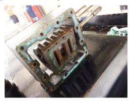
This all sits in the conventional slide valve type steamchest, very odd. We started by taking out the valve setting blanks and pushing the engine along. This confirmed the timing was in fact correct, so it had to be the piston valve assembly seal on the the cylinder block. Sure enough removing the steamchest and valve assembly revealed a gasket with the bar between one cylinder end and the exhaust port missing. The hunt was then on for a new bit of gasket paper to make a repair.
